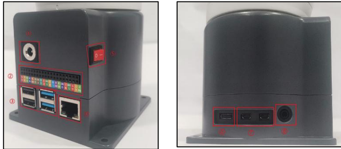
Figure 5.3: The front interface and the left side of the base, where the Raspberry Pi is housed [18]
