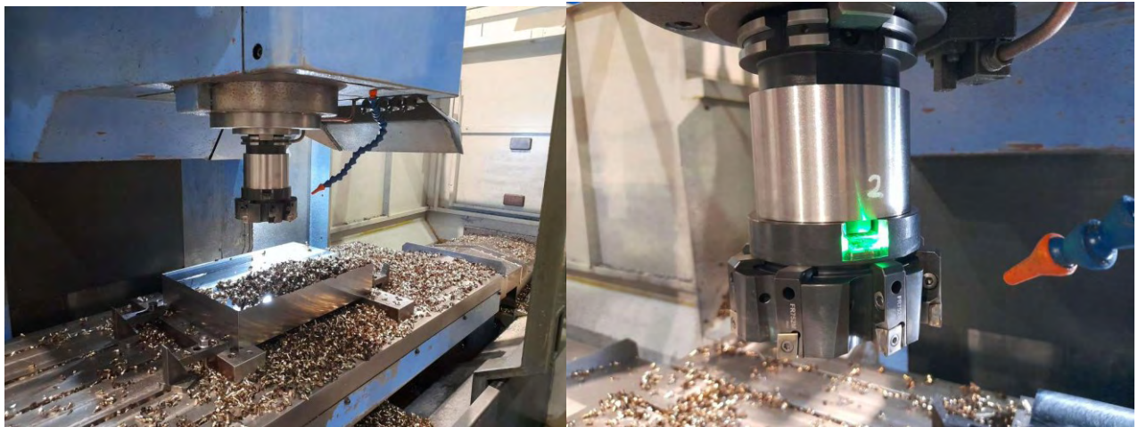
Figure 4.13 The instrumented milling head installed on the Mazak machine tool
