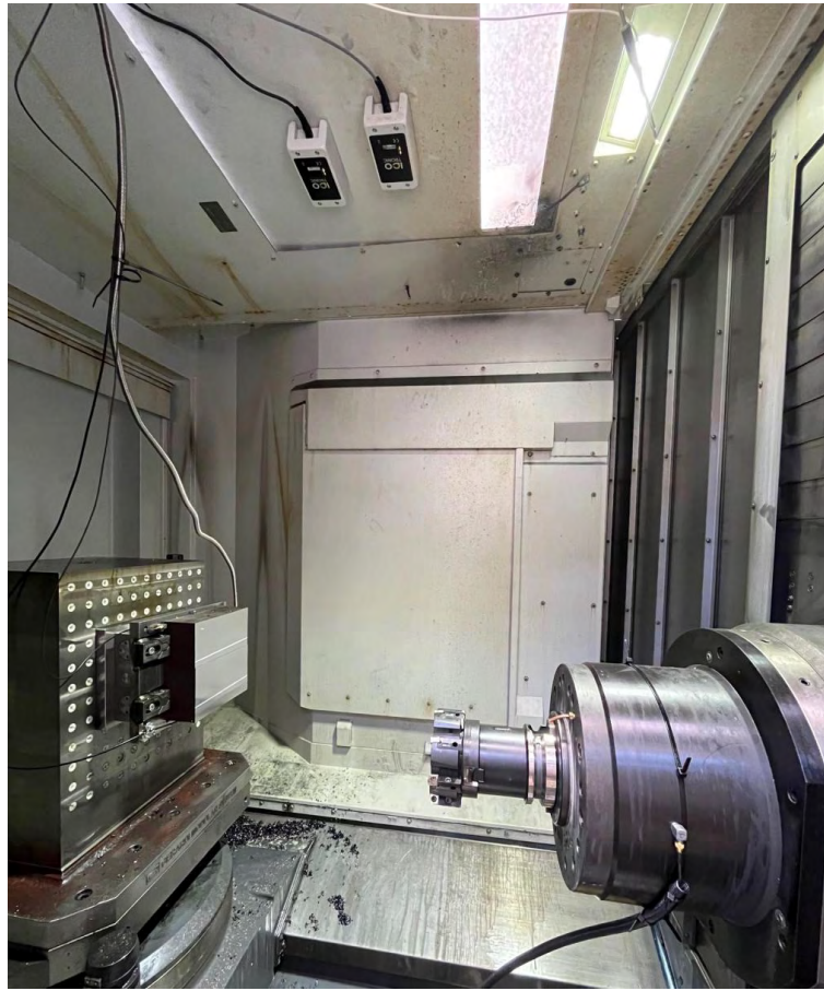
Figure 4.26 The instrumented milling head installed in the Mori Seiki machine tool
