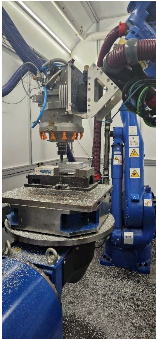
Figure 2.37 Machining of the coupon for the optimized case
