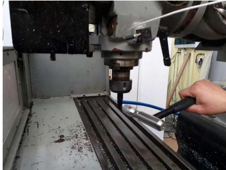
Figure 3.4 Testing of a machine tool with an impact hammer [3.7]
