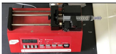
Figure 6.2 Electrospinning system used for the productions of the PCL/PVA vessels.
