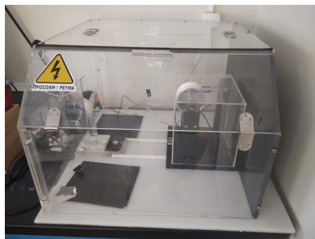
Figure 6.2 Electrospinning system used for the productions of the PCL/PVA vessels.
