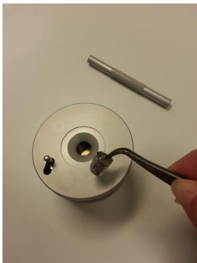
Figure 44: The silver capsule where the samples are placed and measured by the elemental analyzer.
