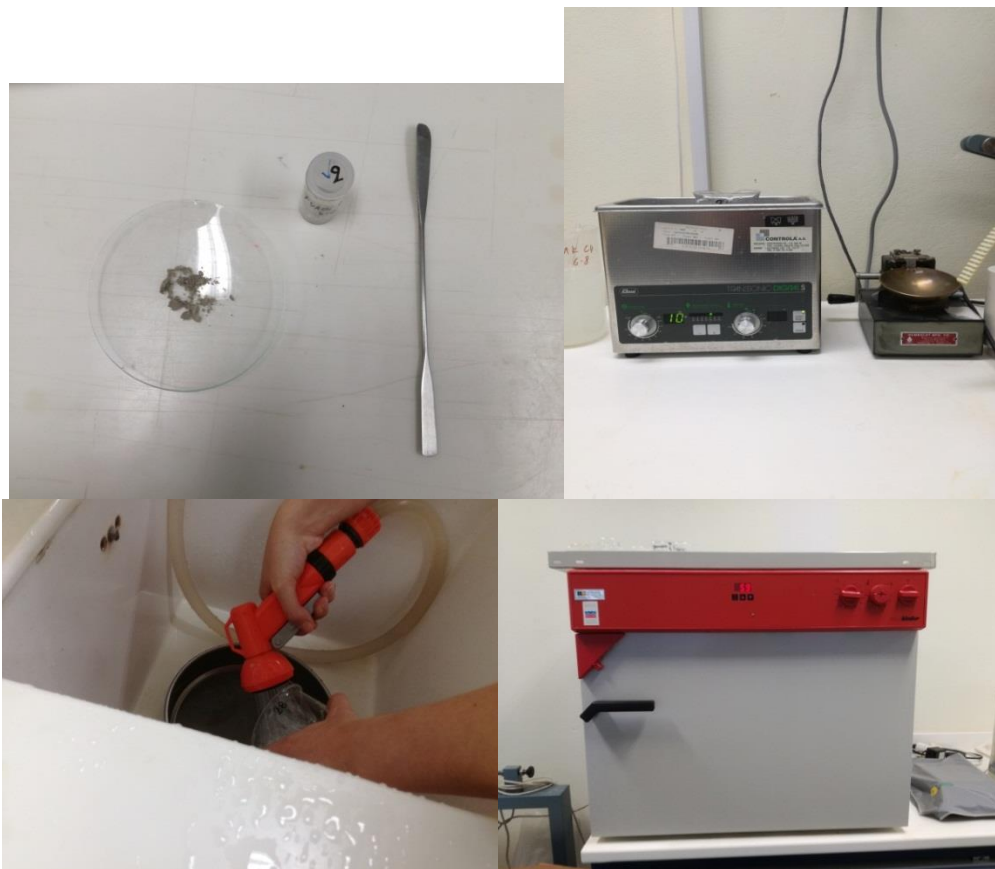
Figure 22: The process that was conducted in all samples in order to be ready for the observation and identification of the foraminifera through the microscope. Up left: A descent amount of sediment was taken from each sample. Up right: It was placed for a few minutes in the ultrasound device. Down left: It was sieved for a +4\phi diameter. Down right: Then it was left overnight in the lab oven at around 55^{\circ}C .
