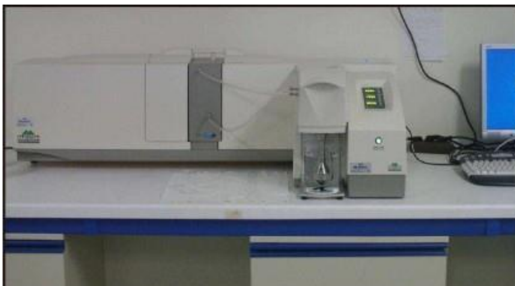
Figure 18: The Malvern Mastersizer 2000 Hydron particle size device that was used for the purpose of this study.
