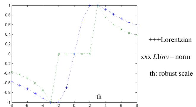
Fig. 1. The Lorentzian and  $L_{linv}$ -norm  $\psi$ -functions aligned and scaled. The direct comparison of the two error norms in rejecting outliers now can be performed.
