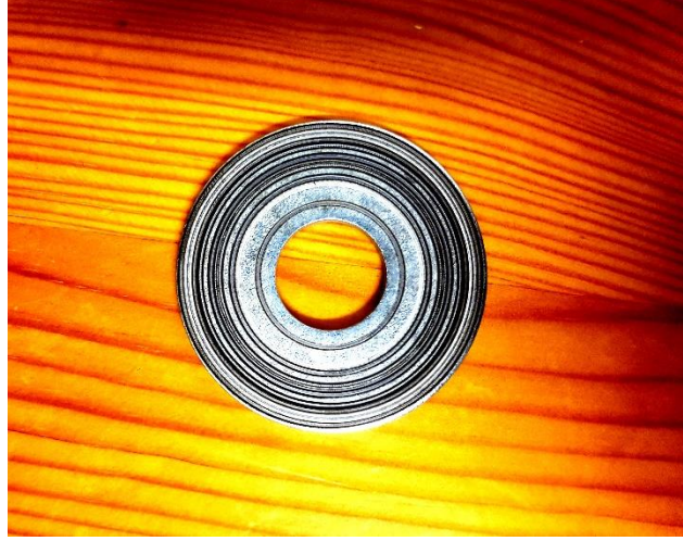
Fig. 6.7: Photograph of the metal plate used for the evaluation of the 3-level implementation of the transducer prototype based on laser ablation. The grooves formed by the material removal are apparent.
